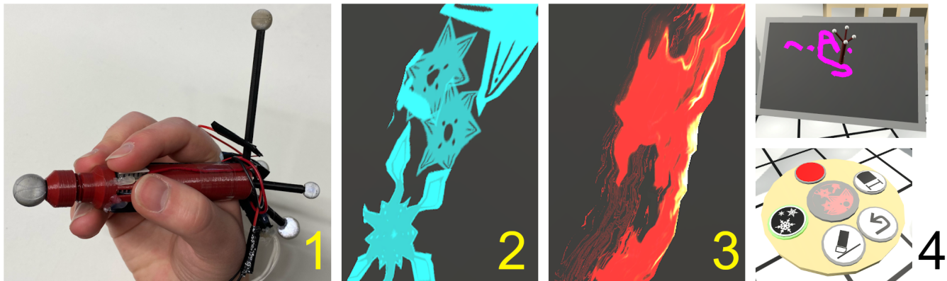
Figure 1: 1) ThermalPen, 2) Snow Blue texture - Cold, 3) Flame Red texture - Hot, and 4) Views of the 3D sketching application, a user sketching (top) and the menu to change color and textures (bottom)
